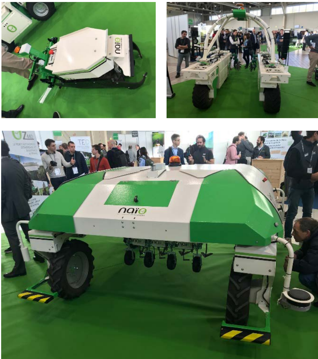
Figure 2. Robotic solutions developed by Naio technologies; eeding robot OZ (upper left image), vineyard robot TED (upper right image) and vegetable robot DINO (lower image).
