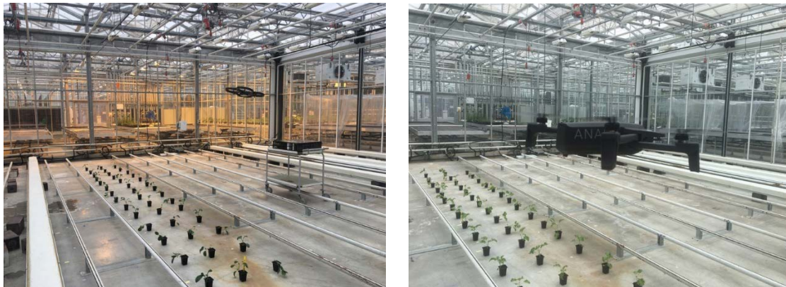
Figure 2. AR.Drone and ANAFI flying in a greenhouse while detecting and counting plant leaves.
