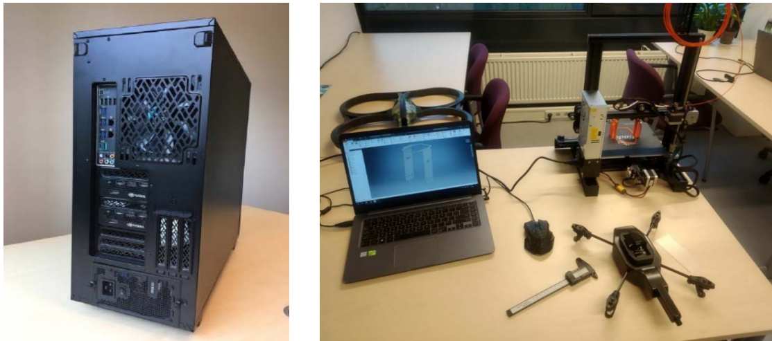
Figure 4. High-performance computer with a Intel Core i9 (3.3 GHz), 2 NVIDIA TITAN RTX, HDD 3TB Samsung 860 EVO, 64 Gb memory RAM, and a Corsair AX1600i board (left) and Creality 3D® Ender-3 DIY 3D printer kit with a 220x220x250mm printing size (right).
