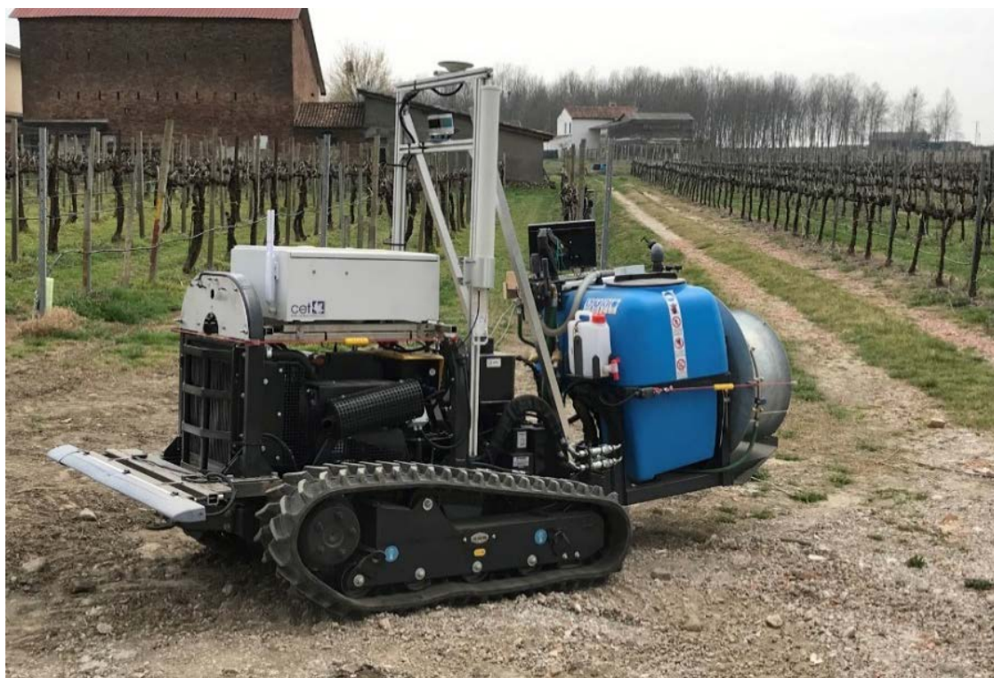
Figure 5. ROVITIS by dr. Giorgio Pantano - a completely autonomous platform that drives by itself from the garage to the vineyard, autonomously completes its operation in the vineyard and returns to the garage.
