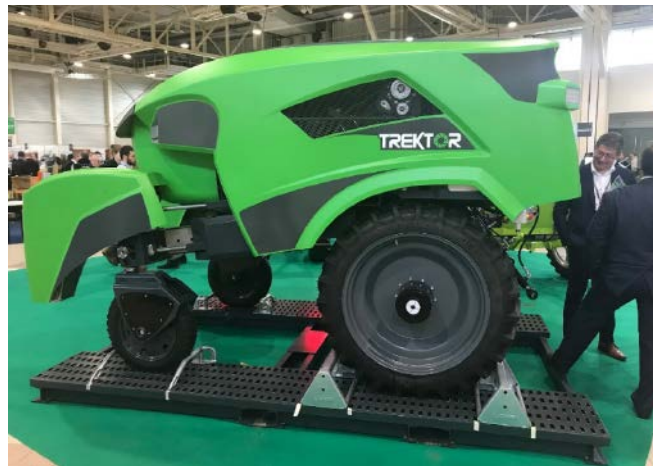
Figure 3: An example of a hybrid robot - Trektor developed by SITIA.
