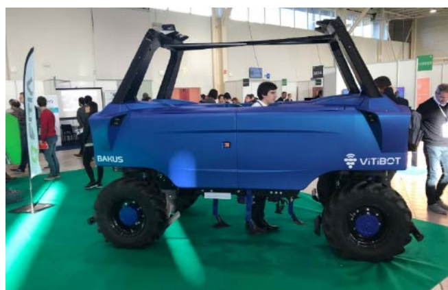
Figure 4. An example of a fully electric platform - ViTiBOT developed by BAKUS.
